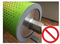
Make sure to put the sleeve centrally on the cylinder
