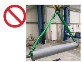
this way you will not install the "roller" on the holder, but you will damage the rubber surface!
